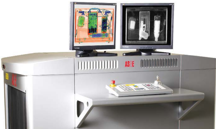
The electronic clutter in the dual-energy transmission image ( left monitor ) obstructs views of the threats in the briefcase. The Z Backscatter image ( right monitor ) of the same briefcase exposes the Glock handgun and plastic and liquid explosives.
