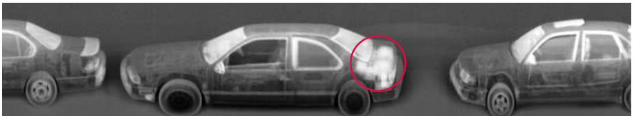
This Z Backscatter image reveals explosives hidden in the trunk of a car (circled in red). The ZBV's continuous screening capability allows security officials to quickly scan unattended lines of vehicles.
