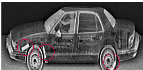
Forwardscatter X-ray image ( top ) with shielded nuclear threat circled in red; Z Backscatter X-ray image ( bottom ) with organic materials circled in red.
