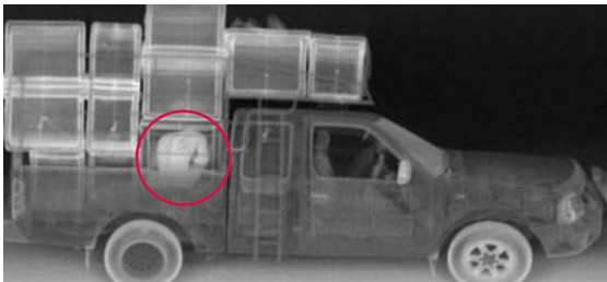
Attempted human smuggling was revealed using the ZBV's safe Z Backscatter technology.
